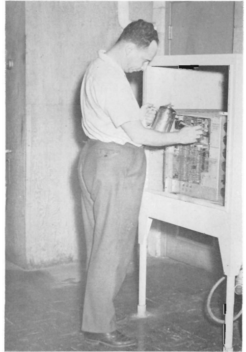
Al DeNeve, service technician at Chicago, spray-cleans a 524B which was turned in for maintenance.
